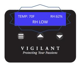
The Guardian control is equipped with several alarms. When in alarm the display brightness and alarm message will flash. All alarms will automatically clear once the condition is corrected.
